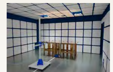
Anechoic chamber of EMC laboratory at Hirose Electric Headquarters
